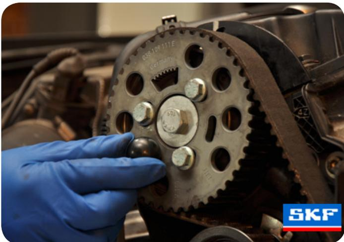
1. Remove the crankshaft pulley cap and timing cover upper case.
