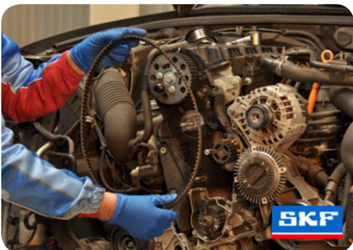
5. Slacken the tensioner nut and turn the tensioner anti clockwise using the correct tool.
