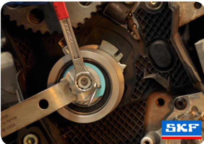
**7.** Undo the camshaft sprocket bolts and turn the pulley, aligning the bolts in the middle of the oblong holes.
