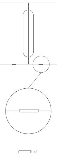
Small transparant plastic parts, to protect the floor.
