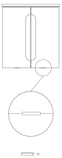
Small transparant plastic parts, to protect the floor.
