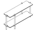
Screw the adjustable feet into the bottom legs and attach the threated rod in the other end
