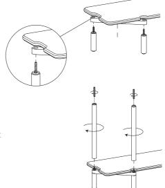
5 Attach the middle legs and insert a threated rod in the other end
