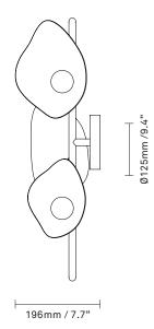
Florii 3 Wall is an oblong wall lamp that gracefully unfolds into three petals from where an integrated LED light softly diffuses.
