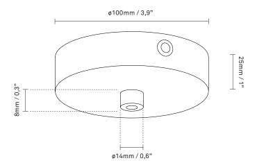
Canopy 1 is an optional accessory for lamps that are delivered without a ceiling plate.
