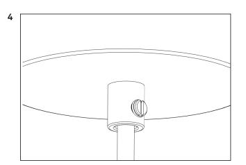
Gently fasten the screw clockwise to the cable to fixate the canopy.
