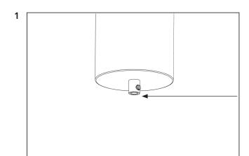
Loosen screw counterclockwise so the cable can pass.
