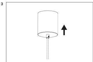
When the lamp is mounted properly to the celing, slide the canopy to the celing.
