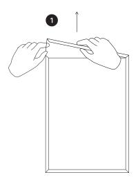
To open the Frame, pull one of the corners apart and remove the rubberband.
