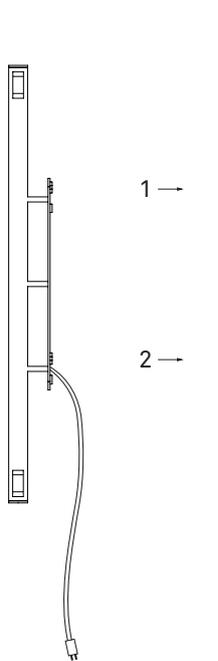
first screw the top hole, than continue with the bottom hole
