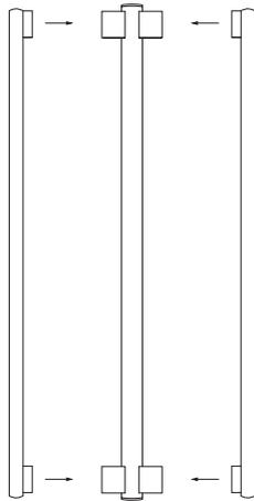
insert each bulb parallel (90°) to the Eiffel frame
