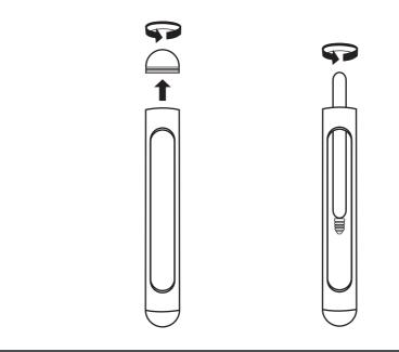
3. Unscrew the lid from the lamp by turning it reversely.
