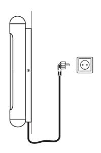
Plug the socket into a power outlet. If there is a built in lamp socket in the wall, the lamp can also be mounted directly to the wall without the cable.
