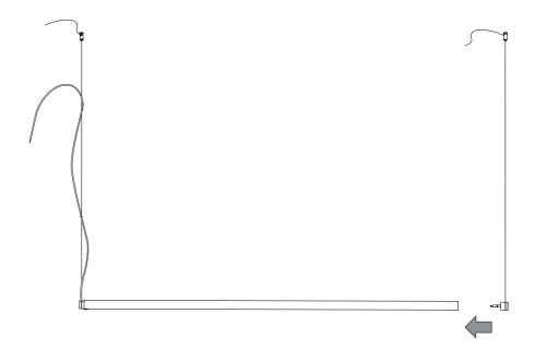
Level the lamp by adjusting the suspension wires. Pull the wire to shorten it or press the tab of the suspension mount to release it. A spirit level can be used to ensure the lamp is hanging perfectly level.
