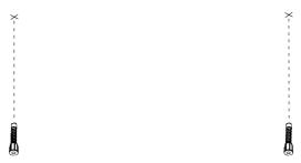
Fix the suspension mount to the ceiling using the provided screws. Disassemble the suspension mount as shown below and insert each screw into the suspension mount, screwing them firmly into place.
