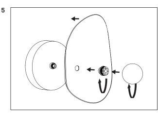
Assemble the rest of the lamp by placing the lamp shade over the base. Then lock it in place by screwing the light source on.
