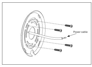
For hardwired installation place bracket over power cable.
