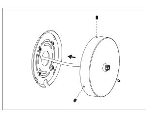
Lock the base in place by tightening the three setscrews with the included hex key.
