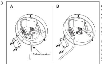
A: For surface mounted cable break out opening in lamp base with a plyer. Secure the cable by clamping it with the strain relief.
