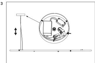
Adjust the cable and wire length close to the lamp's final position.
