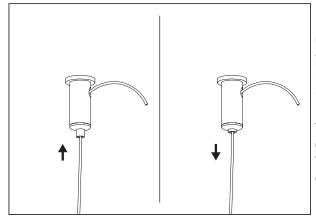
Use the wire lock on the canopy and the ceiling to adjust the lamp to its final position. It is recommended to use a spirit level.
