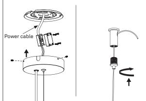
Connect cable ends to the cable terminal. Match the brown wire with "L" and the blue with "N".
