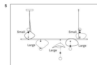
Attach the shades by placing them over the threaded base and lock them in place by screwing a light source on.
