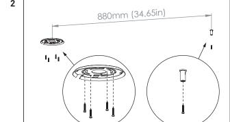
Mount the bracket and ceiling console on the ceiling with screws.
