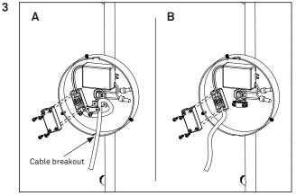
A: For surface mounted cable break out opening in lamp base with a plyer. Secure the cable by clamping it with the strain relief.
