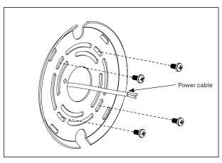
Mount the bracket on the wall or ceiling with screws.
