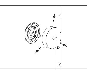
Lock the base in place by tightening the three setscrews with the included hex key.
