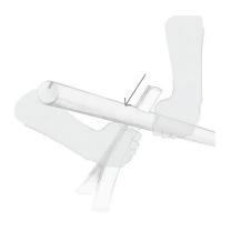
5. Keep the legs(1) pressed together, and insert them into the angled slots in the bar(3).
